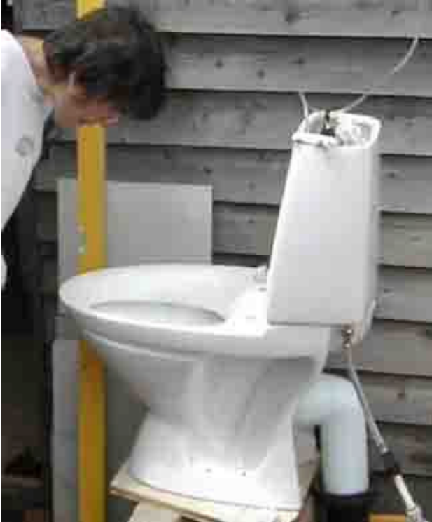
Photo2. An experiment to see how noticeable valve leakage is at different leakage rates.
